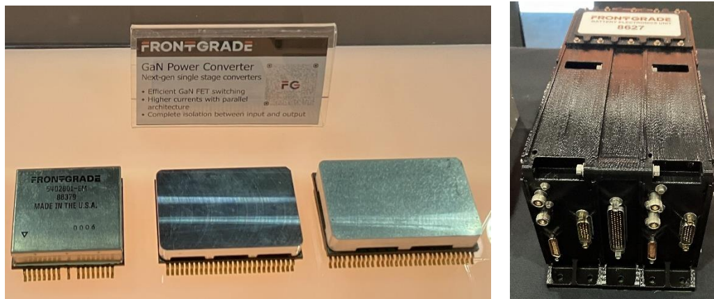
Fig. 17. The Frontgrade single-stage dc-dc converter (shown on the left) is an efficient isolated stepdown regulator rated at 50 to 72 W. The Frontgrade Battery Electronics units like the 8627 (shown on the right) provide autonomous, dissipative, and continuous cell balancing to maximize available battery capacity.
