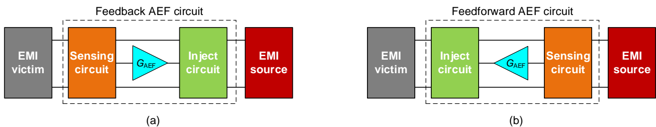
Fig. 5. The sensing, gain and injection stages of an AEF. The control structure could be feedback with high gain (a) or feedforward with unity gain (b).
