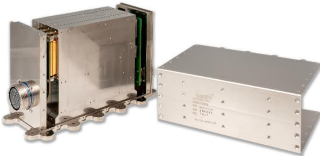
Fig 1. The SGRBX series is a configurable, rad-hard "box solution" that contains four SGRB series dc-dc converters employing GaN technology. The individual SGRB slices are configured within the box framework to deliver up to 1600 W of output power. Customers may select different SGRB series units to be paralleled inside of the box solution to reach the desired output voltages and power levels required for their specific application. If even higher power levels are needed, multiple SGRBX boxes can be paralleled.
