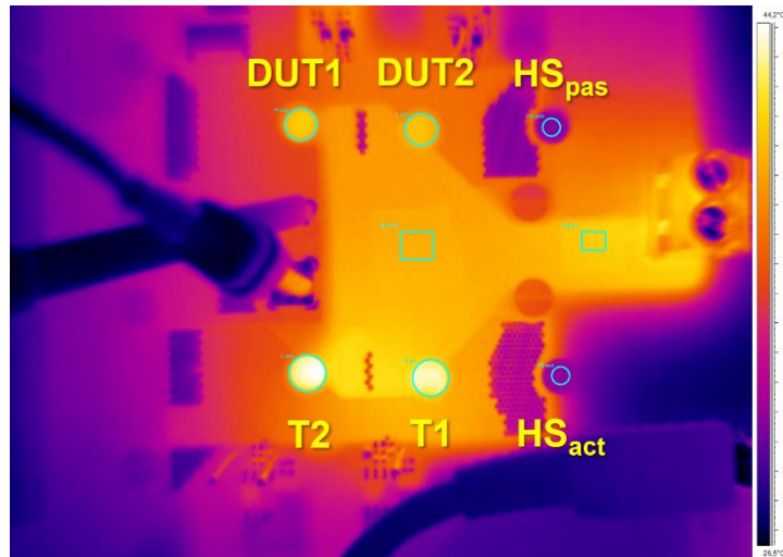
Fig. 3. The temperatures of all six components of interest are measured during operation of the active half bridge (T1 and T2) to determine the C_{oss} losses associated with the passive bridge (DUT1 and DUT2).
