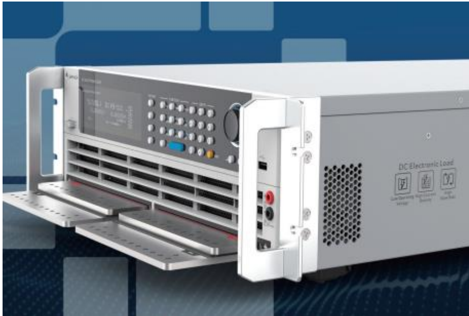
Figure. The Chroma 63202A-20-2000 ultra-low voltage dc electronic load is designed for applications of 2000 A at 0.2 V and 1000 A at 0.1 V, such as simulating loading characteristics of AI microprocessors.
