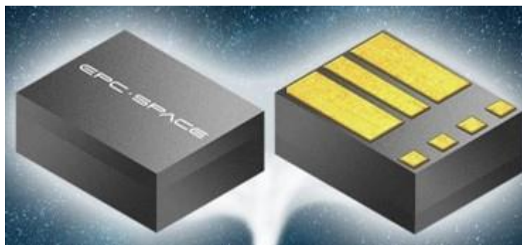
Figure. The 50-Vdc, 6-A EPC7011L7SH is being introduced as the "world's first rad-hard GaN power stage IC". Input logic interface, level shifting, bootstrap charging and gate-drive buffer circuits along with 14-mΩ eGaN output FETs configured as a half-bridge (a) are integrated within a monolithic chip in a custom 7-pin aluminum-nitride SMT ceramic package (b).
