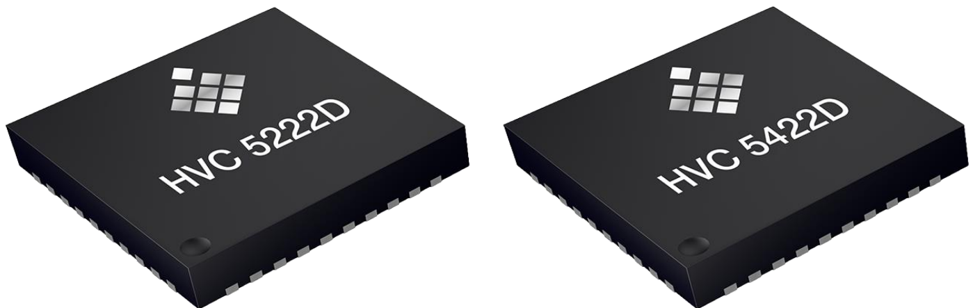
Figure. The HVC 5222D and HVC 5422D motor controllers are capable of 4 x 1-A peak current for driving brushless dc, brushed dc and stepper motors. They feature 4-KB SRAM, 2-KB EEPROM, and either 32-KB ('5222D) or 64-KB ('5422D) flash memory. They are SEooC ASIL B ready according to ISO 26262 to support functional safety applications.
