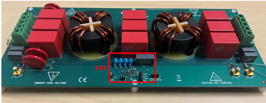
Fig. 11. EVM of a three-phase EMI filter with AEF intended for a 22-kW OBC.
