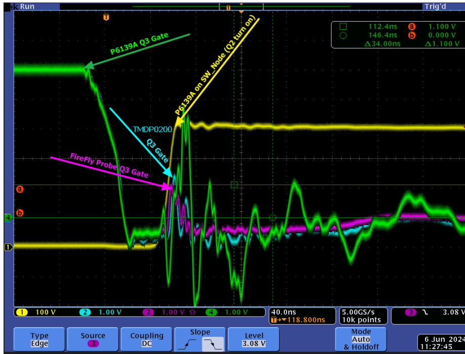
Fig. 21. A three-probe comparison of waveform fidelity.
