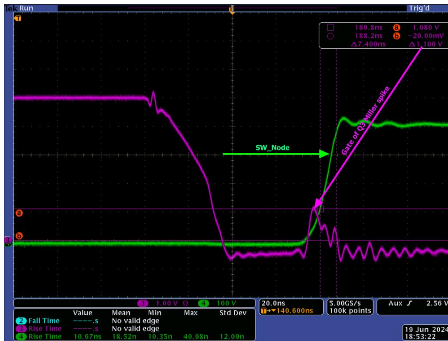
Fig. 22. Real magnitude of Miller spike taken with PMK FireFly optically isolated probe.
