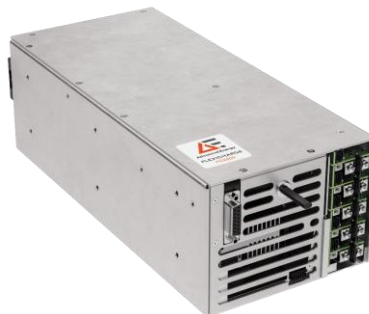
Figure. Delivering up to 3300 W of total power, the FC2500 is a high-voltage 2.5-kJ capacitor charger and low-voltage power supply in one package. It serves as a power supply for laser, IPL and electrosurgery systems, saving size, weight and development time and enabling faster patient treatment through faster charging.
