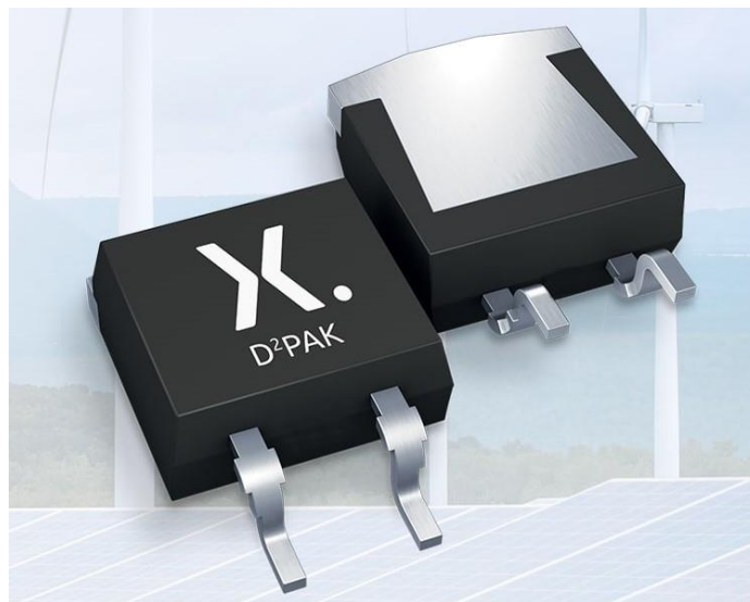
Figure. By removing the middle pin, the D 2 PAK Real-2-Pin package configuration increases pin-to-pin distance from 1.25 mm to over 4 mm, allowing rectifiers to comply with higher creepage and clearance standards as required in high-voltage automotive applications.
