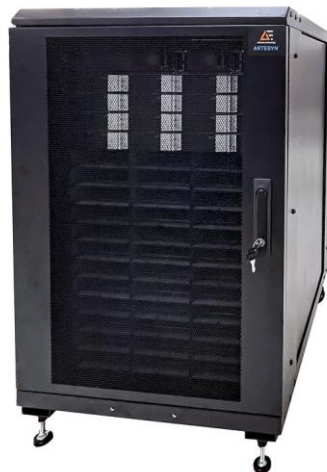
Figure. The LumaDrive Pre-wired Systems series of high-efficiency remote centralized drivers is designed for large-scale horticultural, greenhouse and industrial LED lighting applications. These platforms combine multiple 4-kW modules into a cost-effective pre-wired cabinet that delivers high-density power from 24 kW to 144 kW, while simplifying installation, enabling simple "hot swap" repairs, eliminating extra dimming control connections and reducing the overall cost of any large-scale lighting installation.
