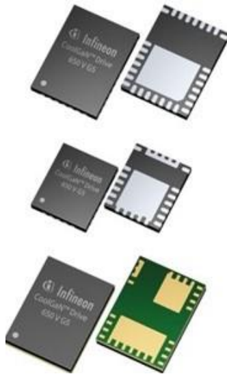
Figure. Infineon's CoolGaN Drive product family consists of single 650-V G5 GaN switches with an integrated gate driver in 5- x 6-mm and 6- x 8-mm PQFNs and 650-V G5 GaN half-bridges with integrated high- and low-side gate drivers in 6- x 8-mm LGAs. These devices enable improved efficiency, reduced system size, and overall cost savings, says the vendor.
