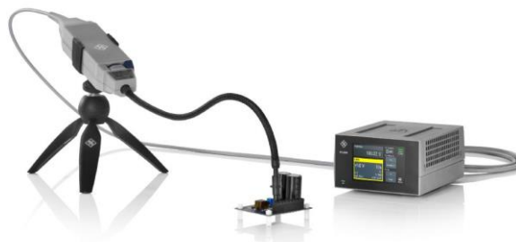
Figure. The R&S RT-ZISO isolated probing system used together with an MXO 5 oscilloscope. The R&S RT-ZISO provides precise differential measurements of up to \pm 3 kV on reference voltages of \pm 60 kV with a rise time of <450 ps and suppresses fast common-mode signals that can distort and interfere with accurate measurements.
