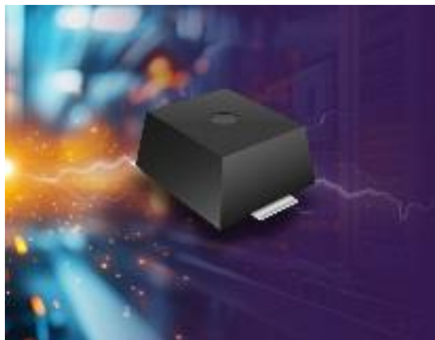
Figure. The PTVS1-240C-M is a high-current bidirectional TVS diode designed for use in high power dc bus clamping applications. This device offers bidirectional port protection with a standoff voltage rating of 240 V. It's RoHS compliant and designed to meet IEC 61000-4-5 8-/20- \mu s, 10-/350- \mu s and 10-/1000- \mu s current surge requirements
