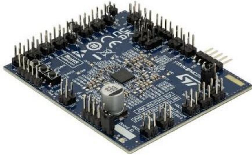
Fig. 3. The STEVAL-PMIC25V1 is an evaluation board for the highly integrated STPMIC25 PMIC. The associated eval kit includes a USB dongle, which provides I 2 C access to the configuration registers of the STPMIC25 device, where voltage settings, power sequences, protection thresholds and other parameters can be set. The board also contains header connectors for external access to the embedded regulators and switches in the device, as well as internal routing via jumpers to satisfy any physical configuration requirements. The passive components on the board are chosen for optimal performance across most use conditions, and three push buttons and digital I/Os allow triggering of the digital controls of the device.
