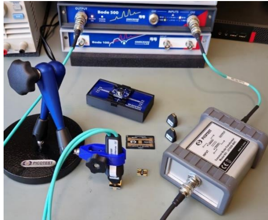
Fig. 2. Two-port shunt through impedance test setup showing the VNA, two-port probe and the common-mode transformer to break the ground loop.
