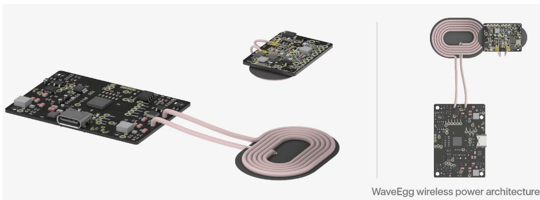
Fig. 1. WaveEgg LP EVB simplifies design and reduces component count for small form factor, cable-free charging of low-power devices up to 6 W.
