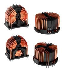
With rated currents from 25 A to 63 A at 60°C and operational voltages up to 600 Vac and 450 Vdc, the chokes are particularly suited for use at frequencies from 10 MHz to 30 MHz. Ensuring cost-effective PCB designs at up to 100 A with forced cooling, the choke is available in horizontal and vertical PCB mounting options to suit specific design requirements. Other features include a broad range of inductance ratings (3 mH to 13 mH), low magnetic leakage flux and superior winding insulation.
