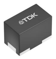
In comparison with the conventional PLEA67B series, whose inductors measure 1.0 x 0.6 x 0.8 mm, the PLE856C series boasts a 40% smaller mounted area and a 50% decrease in volume. The saturation currents are specified between 0.40 A and 0.72 A (typ.).
