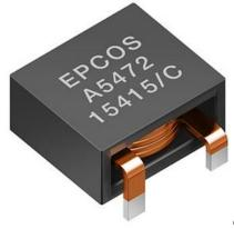
These shielded, through-hole components are designed for saturation currents from 55 A to 120 A at +100°C. The three new types cover a range of inductance values from 1.4  $\mu H$  to 7.2  $\mu H$  and dc resistances as low as 0.46 m $\Omega$  to 1.2 m $\Omega$ . Thanks to the flat-wire winding, the chokes have very compact dimensions of only 33 x 33 mm and a height of 11 mm or 15.3 mm, respectively.
