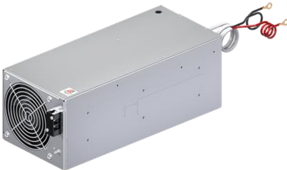
Figure. For use in aesthetic and surgical lasers, the FC4000 4-kJ capacitor charging unit delivers exceptional pulse-to-pulse stability and incorporates an 800-W ac-dc supply with up to 10 isolated outputs for powering system electronics like touch panels, pumps and cooling elements.
