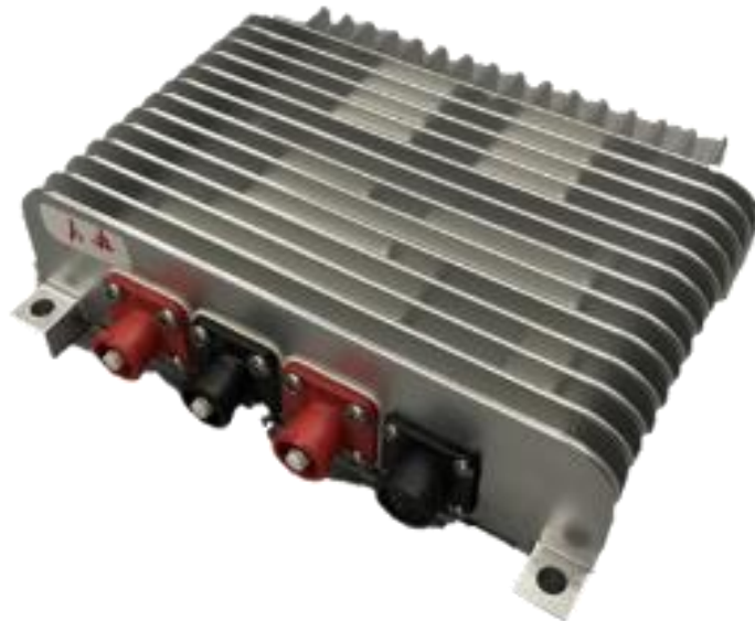
Figure. Measuring 5.57 x 6.97 x 1.75 in. including connectors, the 750-W 48S12.750BCE bidirectional nonisolated dc-dc converter provides a complete solution for in-vehicle power distribution with 12-V/48-V battery configurations for a variety of applications including micro and mild hybrid automotive systems.
