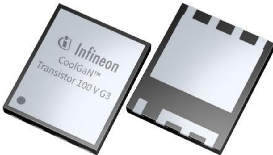
Figure. According to the vendor, the IGD015S10S1 and IGE033S08S1 CoolGaN G3 GaN transistors offer a footprint that, for the first time, allows for easy multi-sourcing strategies and complementary layouts to silicon-based MOSFET designs.
